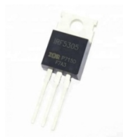
Figure 4: IRF5305 power MOSFET
