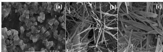
Figure 4: Scanning electron micrographs of the nanostructures that grew at the interface. They were a mix of three prominent morphologies (a) nanocubes (b) nanofibers and (c) nanobelts
