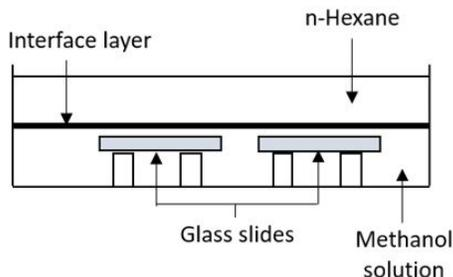
Figure 1: Experimental setup used for seeding. The glass substrates were placed at the bottom of the Petri dish upon glass supports in order to position them closer to the interface layer
