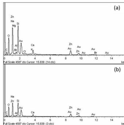
Figure 5: Energy Dispersive X-ray Spectrographs of the ZnO nanostructures grown on (a) glass substrate and (b) n-hexane and methanol interface
