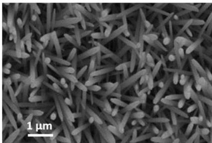
Figure 3: Scanning Electron micrograph showing the top view of the nanorods grown in the second trial
