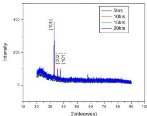
Figure 6: Powder XRD spectra of the ZnO nanostructures for different growth durations: 5 h, 10 h, 15 h and 20 h. Major peaks of wurtzite structure (100), (002) and (101) are indexed and the growth of these planes was found to be prominent in all the samples
