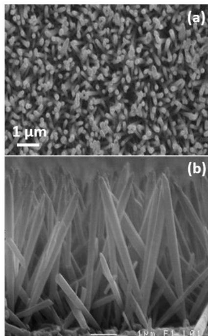
Figure 2: Scanning electron micrographs of the nanomaterial grown on glass substrate during the first trial (a) top view (b) cross-sectional view
